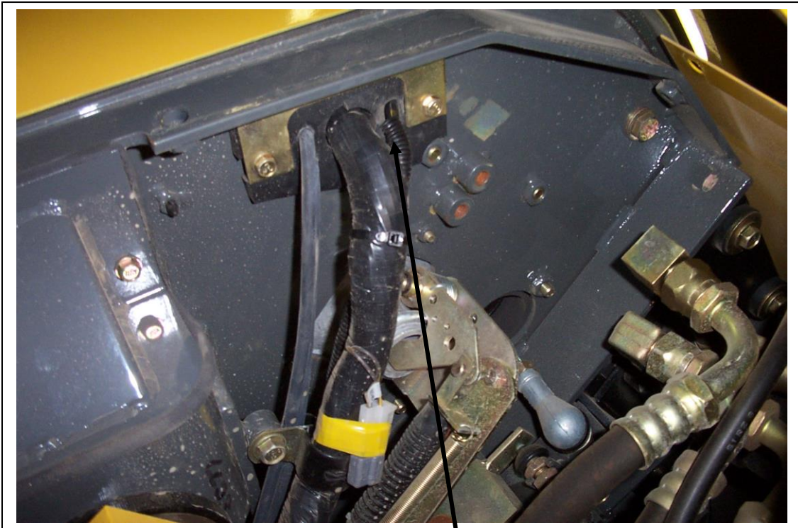
Thermostat knob with all covers back in place.
