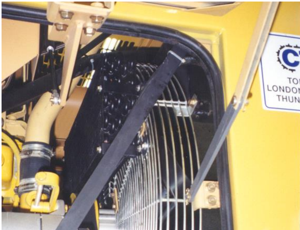
Condenser as viewed from left side.
